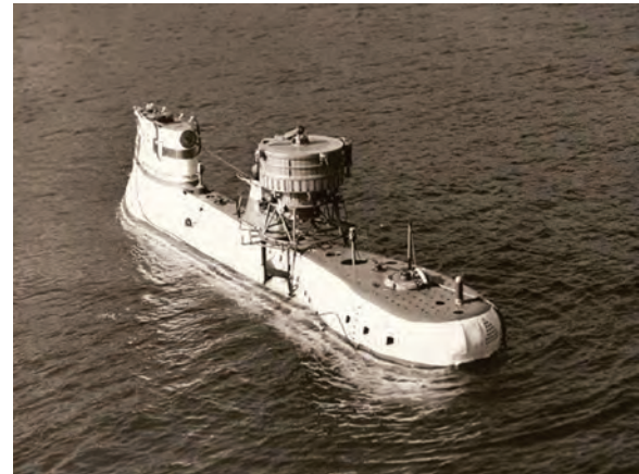
Fig. 2. APU on deck of submersible vehicle
