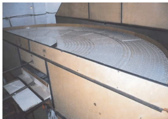
Gas distributor (4,000 mm in diameter) of an industrial ammonia conversion apparatus
