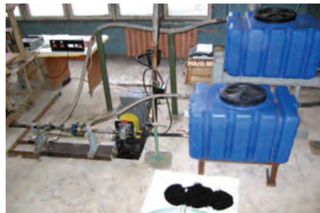
Experimental sample of the cavitation-pulse dispergator to work out the operational regimes with different types of coal.
