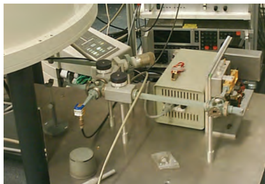
The Stand SQR-110/1 is a quasioptical part of EPR-NMR spectrometer with dynamic nuclear polarization pumping in terahertz frequency band
