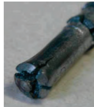
Fig. 1 Brittle fracture without opposite pressure (hardening 10-15 %)
