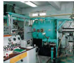
Fig.1 Laboratory plant for pulsed plasma processing, developed at PP NSC KIPT.
