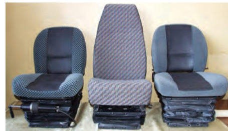
Variants of driver seat designs with autonomous pneumatic vibroprotective modules
