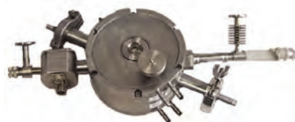
Continuous-flow He-N 2 cryogenic system "UTRECS" C-40 used with optical microscopes for microoptical measurements in the temperature range of 40–1000K. Patent pending in Ukraine.
