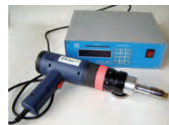
The portable ultrasonic apparatus for hardening and relaxation treatment of welded joints with the power output till 650 W.
