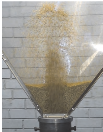
Spouted bed structure (semicircular version, 1:6 scale)
