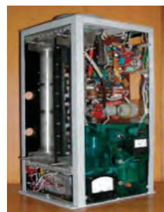
Fig. 2 Glow discharge ozonizer OzWW 4/2
