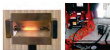
Fig.3. All ceramic IR radiator and their utilization as heater to extra high heat emission in new system for sterilizing treatment equipment
