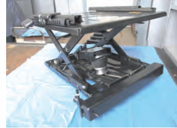
General view of the transport mean driver seat suspension with the autonomous pneumatic vibroprotective.
