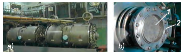
Fig.1 The general view of LINAC (a), and the beam extraction windows (b) - "1" is the window made of CCCM; "2" is the extraction window mounting.
